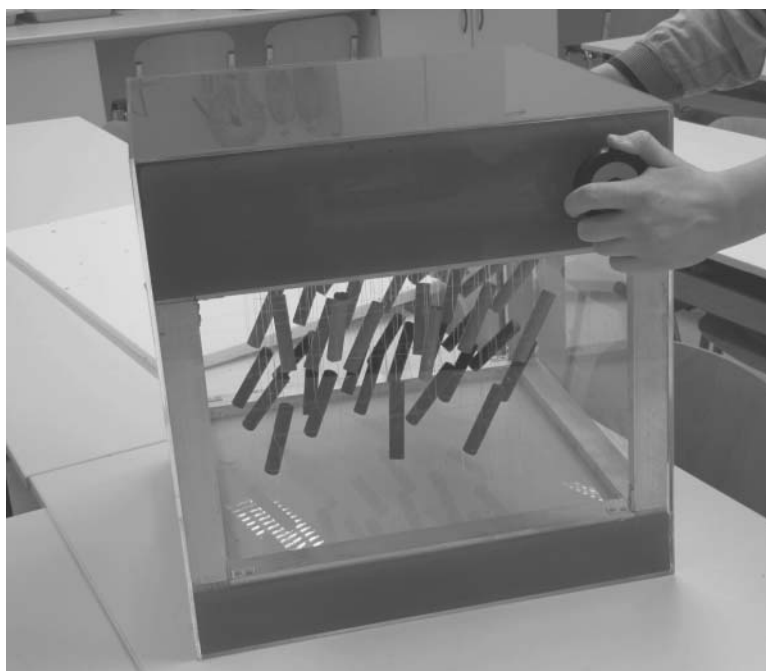
Figure 2. Mechanical teaching tool for presentation of smectic A to smectic C phase transition due to rotation of double handle.
